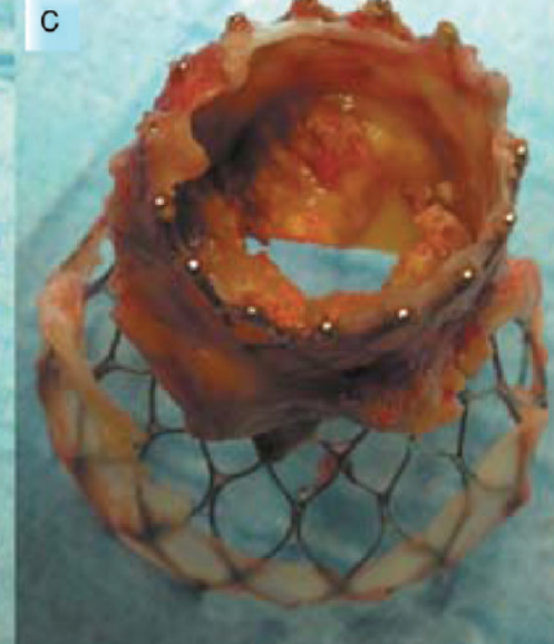
Figure 5 Transcatheter heart valve structural failure. (A–C) Extensive leaflet calcification on the outflow and inflow aspects of an explanted CoreValve. Reprinted with permission from Ong et al. 71
